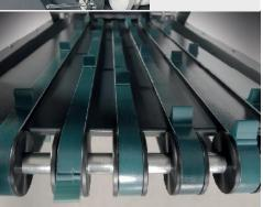
PV40\* is the new automatic bagging machine for garments and constitutes an evolution of its predecessor PV38, with targeted improvements and with a detachable transport belt according to The customer's needs. The output capacity of PV40 depends on the output speed of STP1000 or on how fast the operator places the garments in the machine when the machine functions independently. PV40是新款自动装袋机,是PV38的改进版本,根据客户的要求进行了升级和装配了可拆卸的输送带结构。PV40的产量是由STP1000的输出速度决定的,或者当机器单独运行的时候操作人员单独放入成衣的速度决定。
